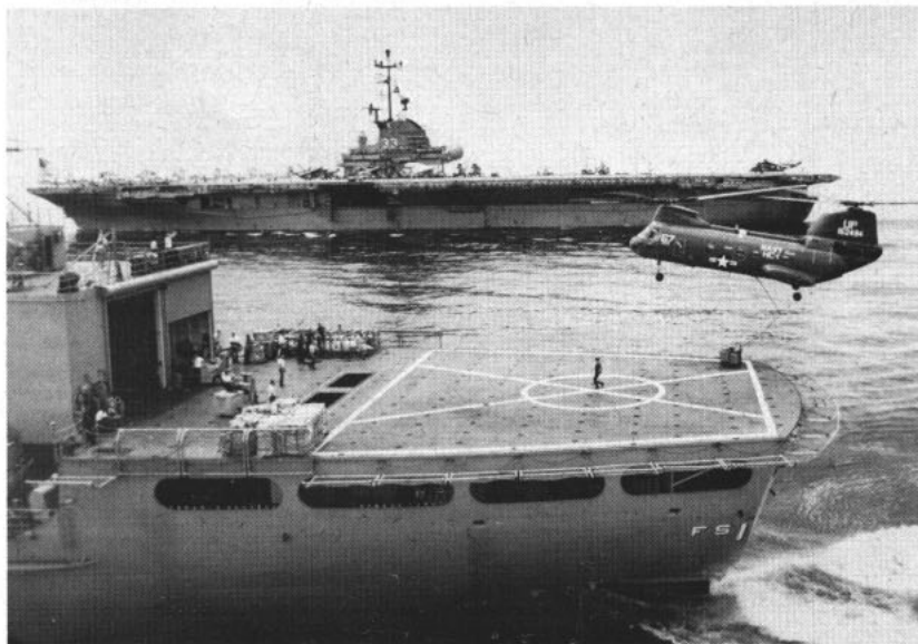
VERTREP AT WORK —Sea Knight helicopter hovers over flight deck of USS Mars (AFS 1) during underway vertical replenishment of USS Kearsarge .
